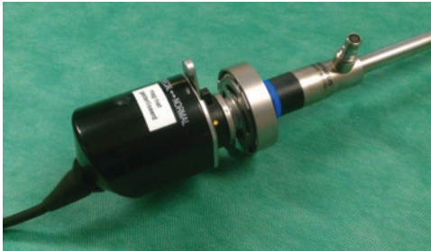
Figure 1. Near-infrared filter attached to rigid 0° conventional laparoscope
